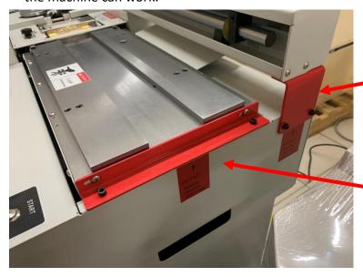
2. Please cut off the cable tie in the right side of the cabinet. This has to be removed too before operation.
